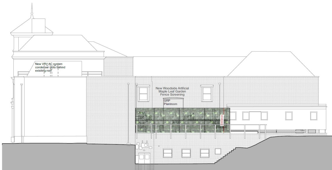
Proposed West Elevation With Plant Screening
